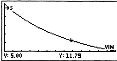
Figure 3-54. “LDO SINK” Calculator Program eases tedious thermal calculations. (See Appendix C).
